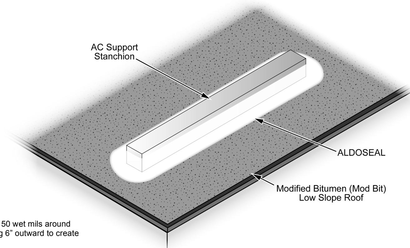
1. Apply a minimum of 50 wet mils around stanchion, feathering 6" outward to create positive drainage.
