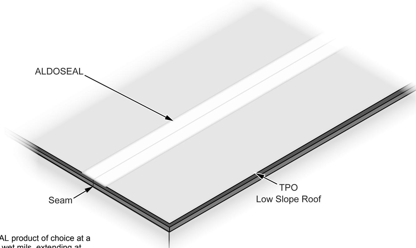
1. Apply the ALDOSEAL product of choice at a minimum rate of 50 wet mils, extending at least 6" on either side of the seam.
